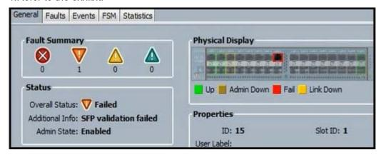
When an engineer inserts 8-Gb Fibre Channel SFP port 15 on a Cisco UCS Fabric Interconnect, the port fails.
