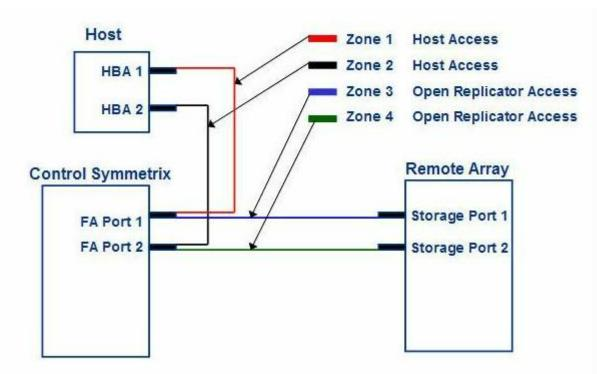
The SAN zones (Zones 3 and 4) shown in the exhibit have been created during an Open Replicator implementation. The control devices in the Symmetrix array are mapped to both front-end ports.
