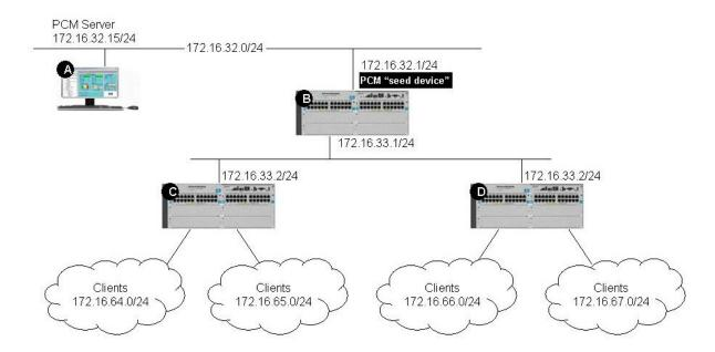
You have installed PCM+ and all of its plug-in applications on this network. You have not performed any additional configuration. How many subnets will be displayed in the navigation tree when you log in to PCM+ for the first time?
